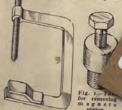
Fig. 2.—Spring compressing tool for removing valve springs in s.h.v. engines.
