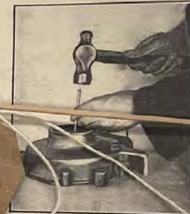
Fig. 6.—Tapping out the old drive side half of valve guide with a hammer and brass drift.
